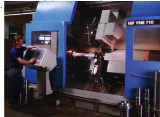
Specializing in single to short runs of larger components. Advance is well-equipped with three state-of-the-art CNC Boehringer turning lathes, the largest of which can handle an 28-inch diameter part up to 8 feet in length between centers.
