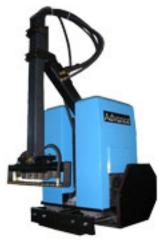
The Advance line of straight-line digital reciprocating sprayers includes the popular SR-1155; its little brother, the SR-1145; and its big brother, the SR-1165. They fit 300- to 1,800-ton DCMs. These feature-laden workhorses have been designed to stand up to rigorous work schedules with minimum maintenance.
