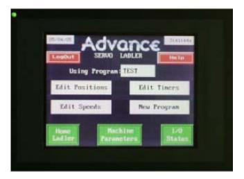
The Advance Servo Ladler operator station uses an easy-to-read color 5.75" LCD.
