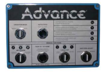
Controls can be set to Manual or Auto by turning a selector switch. A selector switch increases or decreases the shot size.
