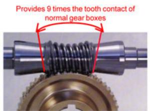
The gear box in Advance's ladlers is either a ground helical gear set or a Cone Drive double-enveloping gear set where the worm is manufactured in an hourglass configuration and wraps around the worm wheel. Either provides low backlash and extremely long life.
